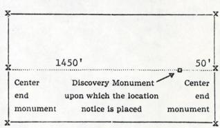
Stone monuments must be three feet high. must be four feet above ground and substantial, no thickness is specified.
